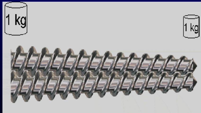
Conical Co-Rotating Screws allow for de-aeration of the mix for maximum product density (Sinking)
